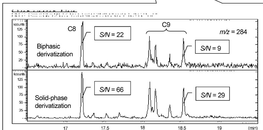
Fig. 3. Total and selected ion chromatograms for analytes in river water.
