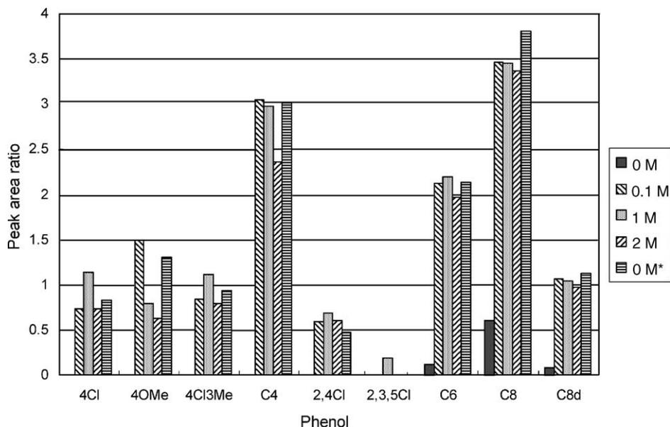
Fig. 2. Effect of NaOH concentration on adsorption of phenols. The peak area ratio of C8d is reduced to 1/100. \*Solid phase was conditioned with 0.1 M NaOH (2.5 ml).
