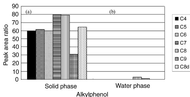
Fig. 1. Recovery of alkylphenols from (a) solid phase and (b) water phase that passed through the solid phase. The peak area ratios of C9 and C8d are reduced to 1/10 and 1/2, respectively.
